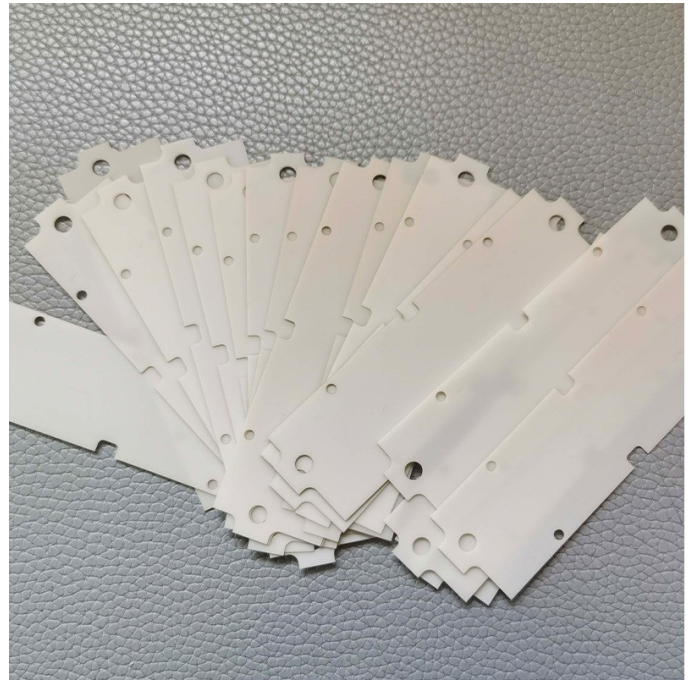
Laser-processed AlN substrates
